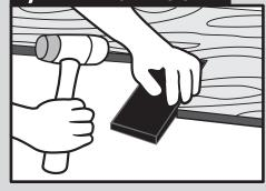
Provides even distribution of hammer force when tapping planks together
